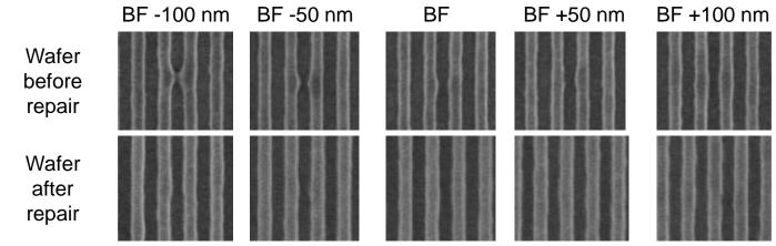
40 nm HP performed on the ASML Alpha Demo Tool
