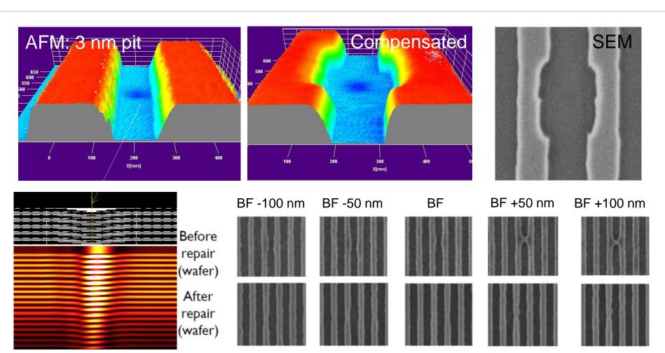
Propagating ML pit simulation Through-focus ML pit compensation repair (see R. Jonckheere *et al.*, Proc. SPIE 8166, 81661G (2011))
