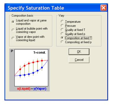
The composition basis for the calculations is specified by the left set of radio buttons. The independent variable is specified by the right set of buttons. Choose one button from each list. A small phase diagram depicts the type of calculation to be performed; this diagram changes as different buttons in the two lists are chosen. The red and blue dots indicate the points to be calculated, and the gray lines connect liquid and vapor points that are displayed in a given row of a table.
