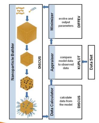
Refined with DIFFEV Au *fcc*: *a*, *u*<sub>iso</sub>(Au) Ligand: surface density, angle with respect to particle face, Au-S distances
