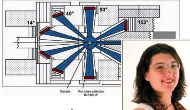
L1: 9m, Qmax=50 Å-1, ∆d/d=0.3 % Typical PDF measurement 3-4 hrs Sample amounts down to 200 mg Ancillary: 4 K-800 K, pressure cell 10 kbar Web based instrument interface Automatic creation of PDF allobet@lanl.gov
