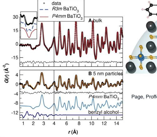
Capping groups observed by scattering for the first time (for any polydisperse nanoparticle system).
