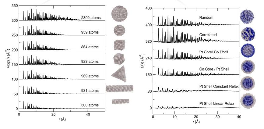
Atomic PDF has indirect sensitivity to size, shape, and architecture of finite materials because it is a distribution of all atom-atom pairs in the scattering volume... this is **a modeling challenge**.
