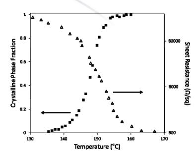
Phase content links to reflectivity, charge transport, *etc.* across amorphous to crystalline phase transition
