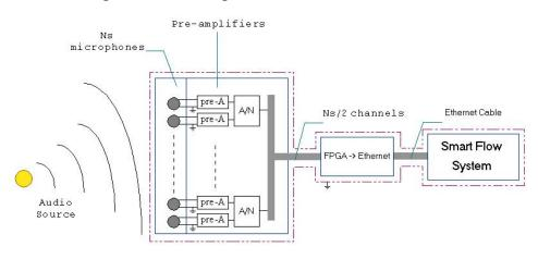
Figure 6: Microphone Array Mark III schematic.
