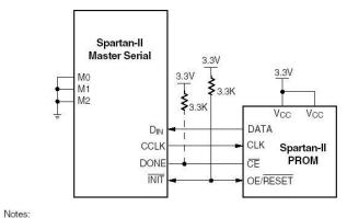
1. If the DriveDone configuration option is not active, pull up DONE with a  $3.3 \text{K}\Omega$  resistor.
