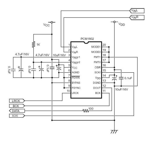
Figure 10: Schematic of the digitalization stage.
