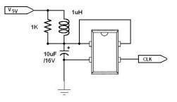
Figure 16: Schematic of the clock stage.
