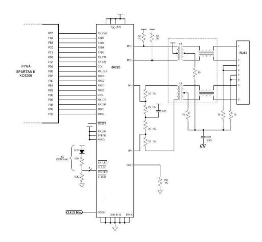
Figure 19: Schematic of the Ethernet stage.
