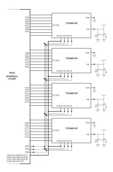
Figure 18: Schematic of the memory stage.
