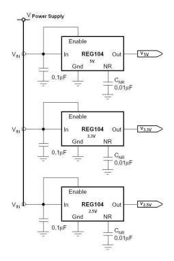
Figure 14: Schematic of the power stage.
