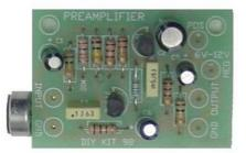
Figure 5: Microphone Array Mark II Preamplifier.
