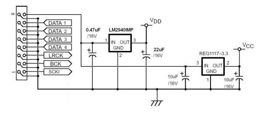
Figure 11: Schematic of the Motherboard connection stage.
