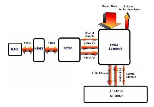
Figure 13: Motherboard schematic overview.
