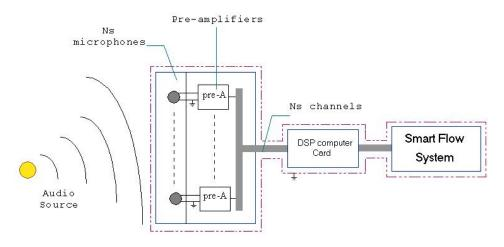
Figure 3: Microphone Array Mark II schematic.
