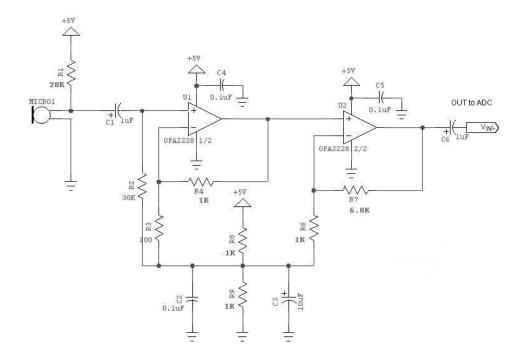
Figure 9: Schematic of the amplification stage for the left channel.
