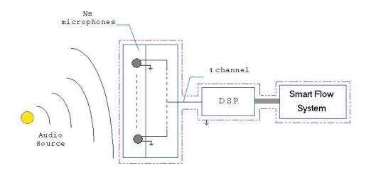
Figure 1: Microphone Array Mark I schematic.
