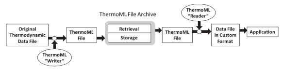
Fig. 2. Global delivery process for experimental thermophysical and thermochemical property data.
