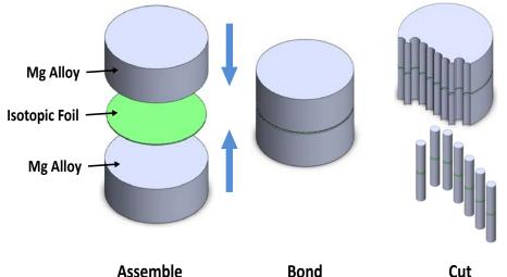
Schematic Mg-alloy sample assembly for high temperature isotopic tracer diffusion measurements using the long capillary method.
