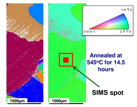
Electron Backscatter Diffraction (EBSD) map (inverse pole figure – top right) of grain orientations in a pure polycrystalline Mg rod after annealing treatment. *left*: Identical grain structure map with enhanced contrast.
