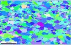
As-extruded microstructure (EBSD), mean grain size ~10 μm, broad distribution
