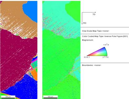
Electron Backscatter Diffraction (EBSD) map (inverse pole figure – top right) of grain orientations in a pure polycrystalline Mg rod after an annealing treatment at 545°C for 14.5 hours. Figure on the top left is the identical grain structure map with enhanced contrast.
