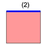
(2) Deposit thin film (100 nm) of stable isotope of an alloy element (e.g., Mg<sup>26</sup>) on annealed sample (3) Anneal at T<sub>o</sub> for desired times (mins to hrs) to cause isotope to diffuse inwards
