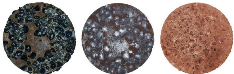
As-tested condition removed from Tank 2      Sonicated for 3 minutes in Deionized Water      Brushed for 4 minutes in HCl/H<sub>2</sub>O Solution
