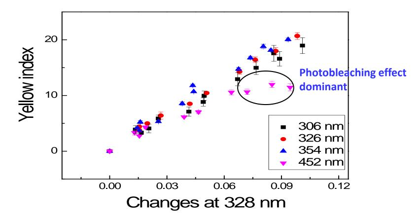
✓ Curves for different wavelengths basically superposed initially (up to about 900 MJ/m<sup>2</sup>), then deviation occurred for 452 nm, implying the photobleaching effect overpassed the yellowing growth then.
