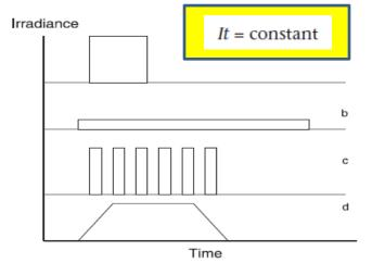
Figure 1—A selection of radiant flux versus exposure time regimes for testing the law of reciprocity in which the dose (integrated area on plot) for each exposure regime is identical. Assuming that the reciprocity law is obeyed, then the photoresponse for each of these exposure regimes should be the same (adapted from reference 6).
