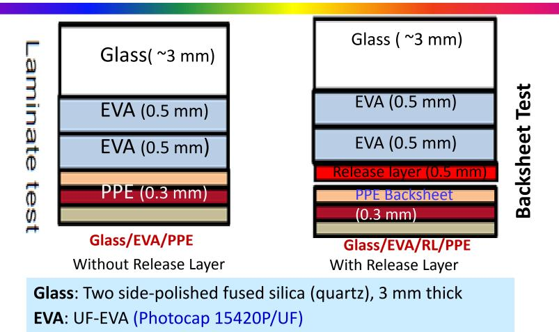
**Release Layer**: FEP film, 500 µm,
