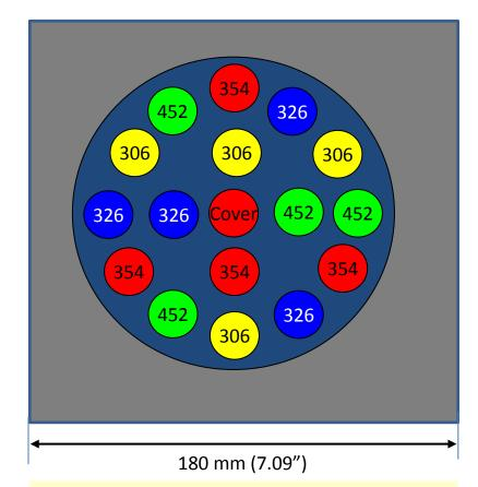
Varying wavelength range with narrow band pass filters,  $(306 \pm 3)$  nm,  $(326 \pm 6)$  nm,  $(354 \pm 12)$  nm and  $(452 \pm 24)$  nm.
