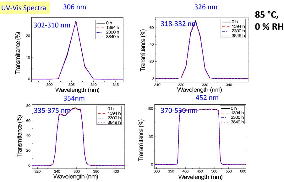
No obvious changes have been observed for these band pass filters at 85  $^{\circ}\text{C}/0$  % RH on the SPHERE so far.
