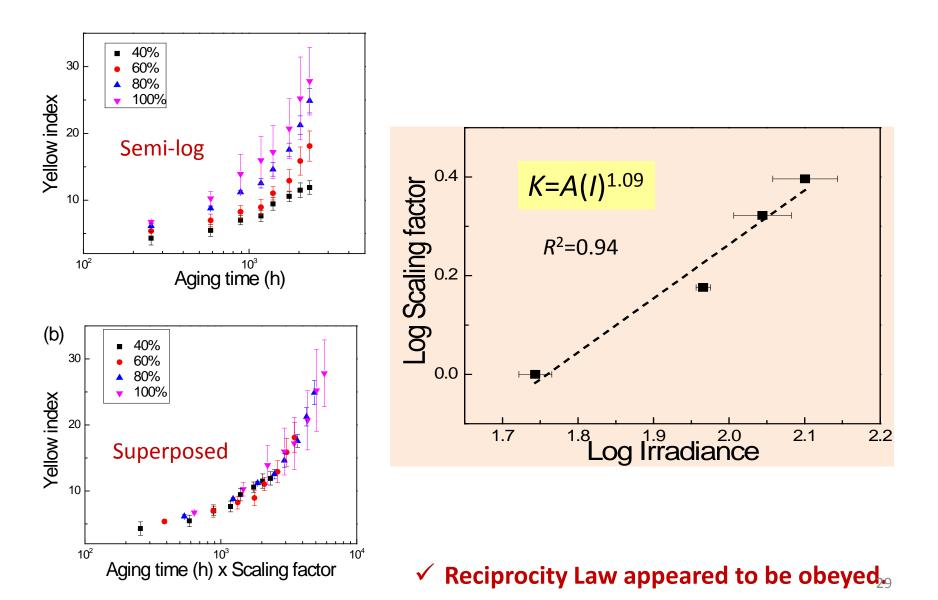
Based on the current exposure data, the Reciprocity Law appeared to be obeyed for the growth of yellowing index of the Glass/EVA/PPE laminated system exposed to SPHERE at 85 °C/dry.
