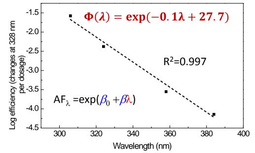
The relative efficiencies of loss of UV absorptions in terms of 306 nm, 326 nm and 354 nm is consistent with those of YI.
