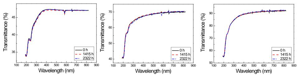
ND filters are essentially stable during UV exposure at 85 °C/dry on the SPHERE so far.
