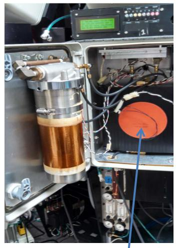
Sample cover with heating pad. The sample is held inside.
