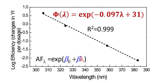
> An exponential dependence between efficiency and wavelength was obtained.
