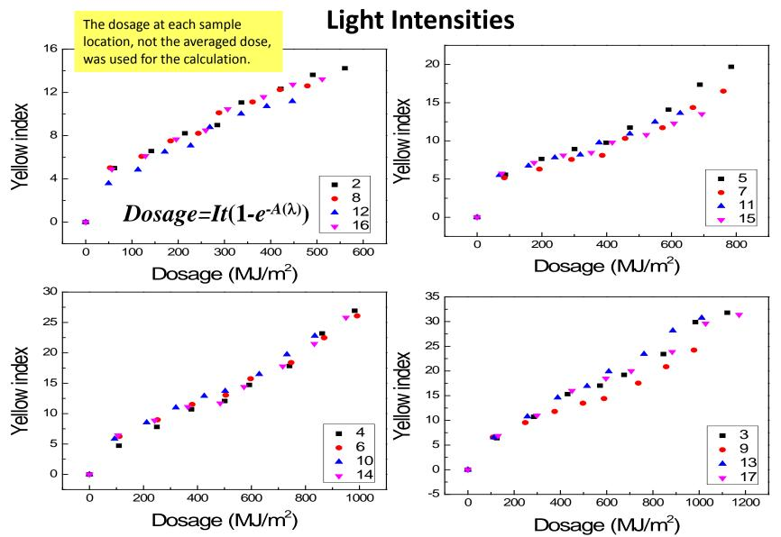
The data from the replicates are generally consistent; the deviation could be due to the non-uniformity of the EVA curing and the EVA thickness. 23
