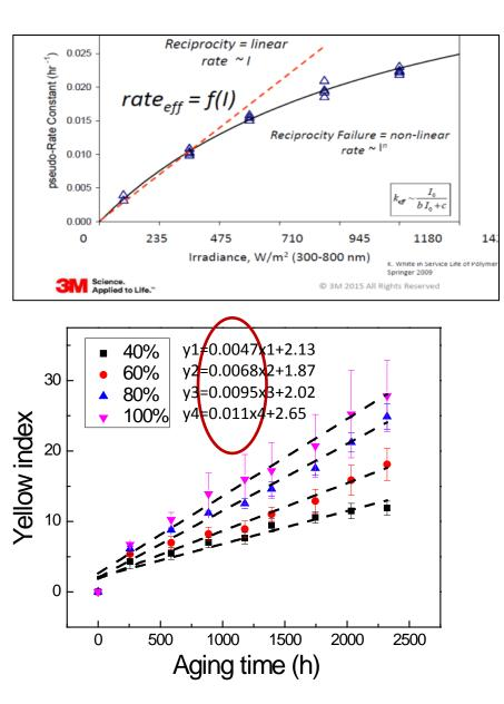
Pseudo-rate constant is defined as the slope of <u>yellow index vs. time</u> curve in this study (Assuming a linear relationship between yellow index and aging time)
