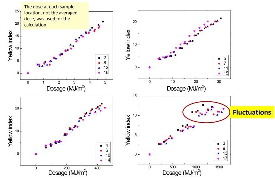
The data from the replicates are generally consistent; the deviation could be due to the non-uniformity of the EVA during curing.
