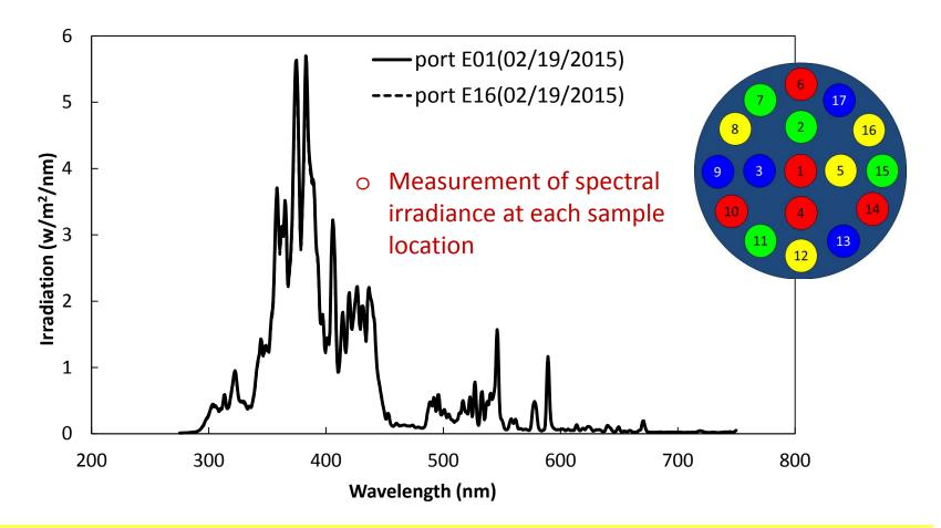
For quantitative study such as reciprocity and action spectrum, the accurate measurement of the spectral irradiance that sample received/absorbed is crucial to the quality of the results.
