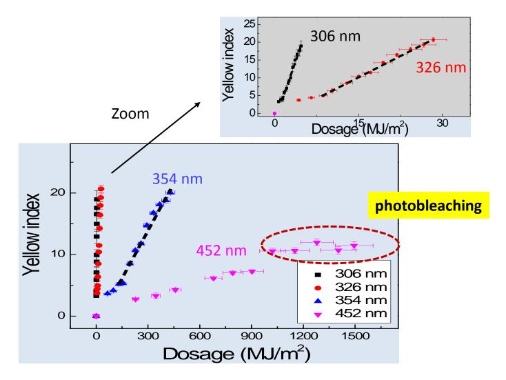
$\checkmark$  Shorter wavelength leads to a higher yellow growth at same dosage. Increase of YI under 452 nm slowed down and then fluctuated at late stage,  $\checkmark$ indicating a photobleaching effect.
