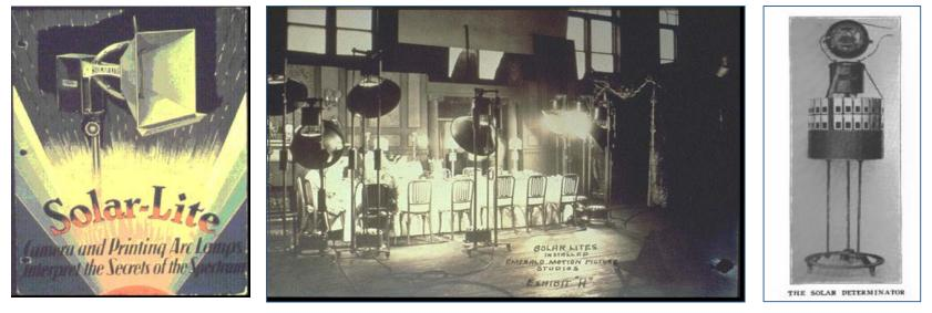
Carbon arc lamps for lithographic plates.
