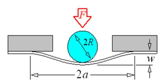
(b) Shaft-loaded blister test (SLBT). A shaft (either flat- or spherically-ended), is driven into the freestanding film, causing delamination. The applied force, F, punch radius, R, blister radius, a, and blister height, w, are used to calculated the interfacial adhesion energy, G.
