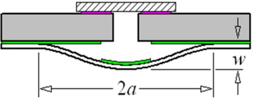
(a) Thermal blister test (TBT). At room temperature, the rear of the hole is covered with a plate, trapping air in the blister cavity. Heat is then applied, causing the air to expand, and driving delamination. Side and top cameras are used to measure the blister radius, a, and blister height, w. These two parameters, along with the pressure of the entrapped air, p, are used to calculate the adhesion energy, G, of the film-substrate interface.
