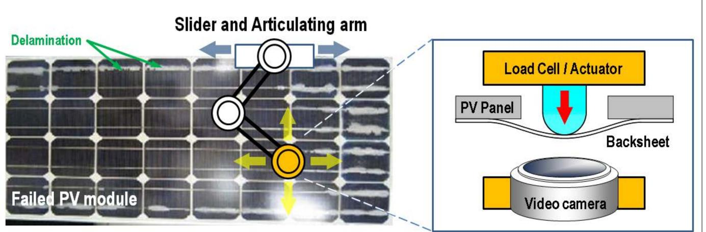
Figure 9. Custom apparatus for blister-testing real, field-weathered PV panel sections, currently being built. The device features an articulating arm that will position a probe for performing shaft-loaded blister tests, anywhere on the panel. Slated completion: QI, 2016.
