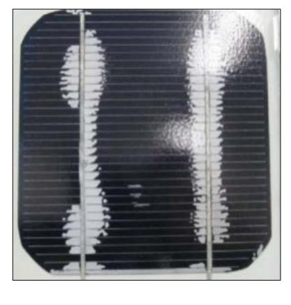
Figure 1. Examples of adhesive delamination in PV panels.
