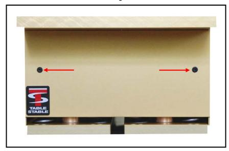
To expose the adjustment nuts, remove the end covers by undoing the screws shown in Fig. 3 (2mm hex key).
