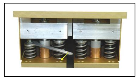
adjustment lf an needed turn the M6 nuts using the spanner provided. Adjust all springs on both sides equally. Moving the spanner to the left raises the units.
