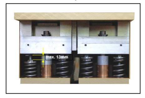
Do not turn the nuts too far or you may damage the units. Under no circumstances should the gap indicated in Fig. 6 be greater than 13mm.
