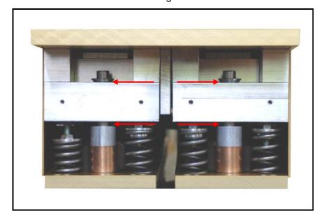
Under load the upper gap and the lower gap shown in Fig. 4 should be approximately equal. (It is however not essential that the gaps be equal - either gap may be as small as 0.5mm without affecting normal operation, but a small subsequent change of load might cause the unit to move against the stop).
