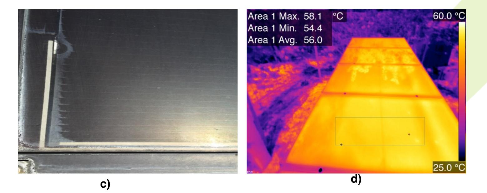
Figure 1. a) Front view of the installation, b) side view of the installation, c) Electro-chemical corrosion, d) Infrared Image
