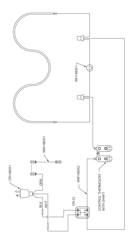
Wiring Diagram • Models PR305215G, PR305210G, PR305225G, PR305220G
