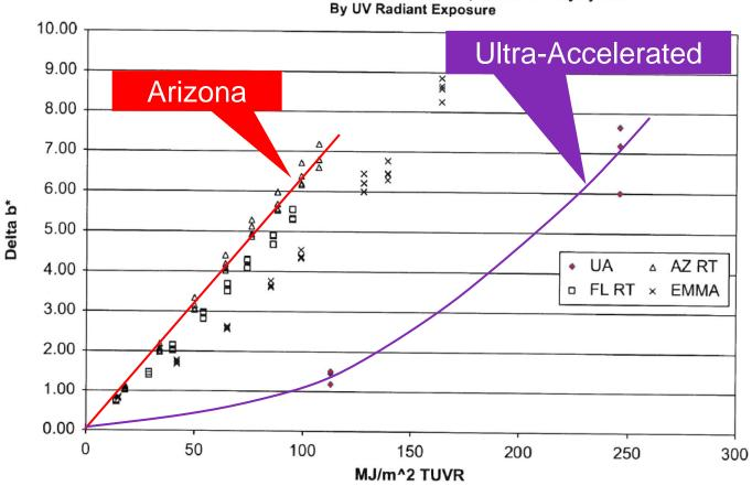
Comparison of FL, AZ, EMMA and UA Exposures of Polystyrene By UV Radiant Exposure
