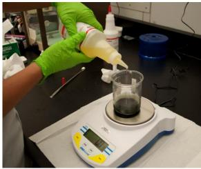
Mix two-part polyurethane and coloring dye. Then vacuum-degas.
