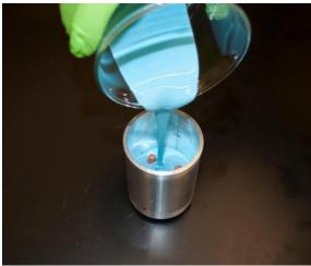
Pouring silicone into replication rig
