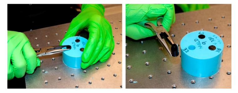
Carefully separate the silicone from the urethane replicas and then remove the replicas with needle nose pliers. The bullet standoff in the replication rig will avoid contact with the striated regions of the bullets, avoiding any damage.
