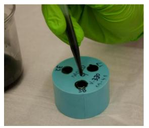
Use a dropper to fill mold with polyurethane. Vacuum-degas again and let cure. 11
