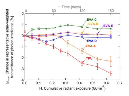
Change in transmittance with radiant exposure (H) for the center of coupons aged with UVA-340 lamps, with the chamber controlled at 60°C and uncontrolled %RH).
