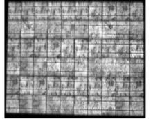
EL image of a panel before 100hr 1000V PID...
