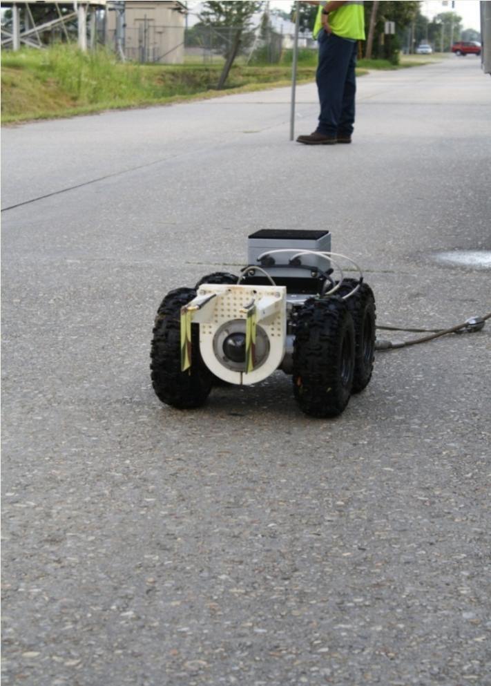
FutureScan Unit Conducting a Pavement Surface Scan
