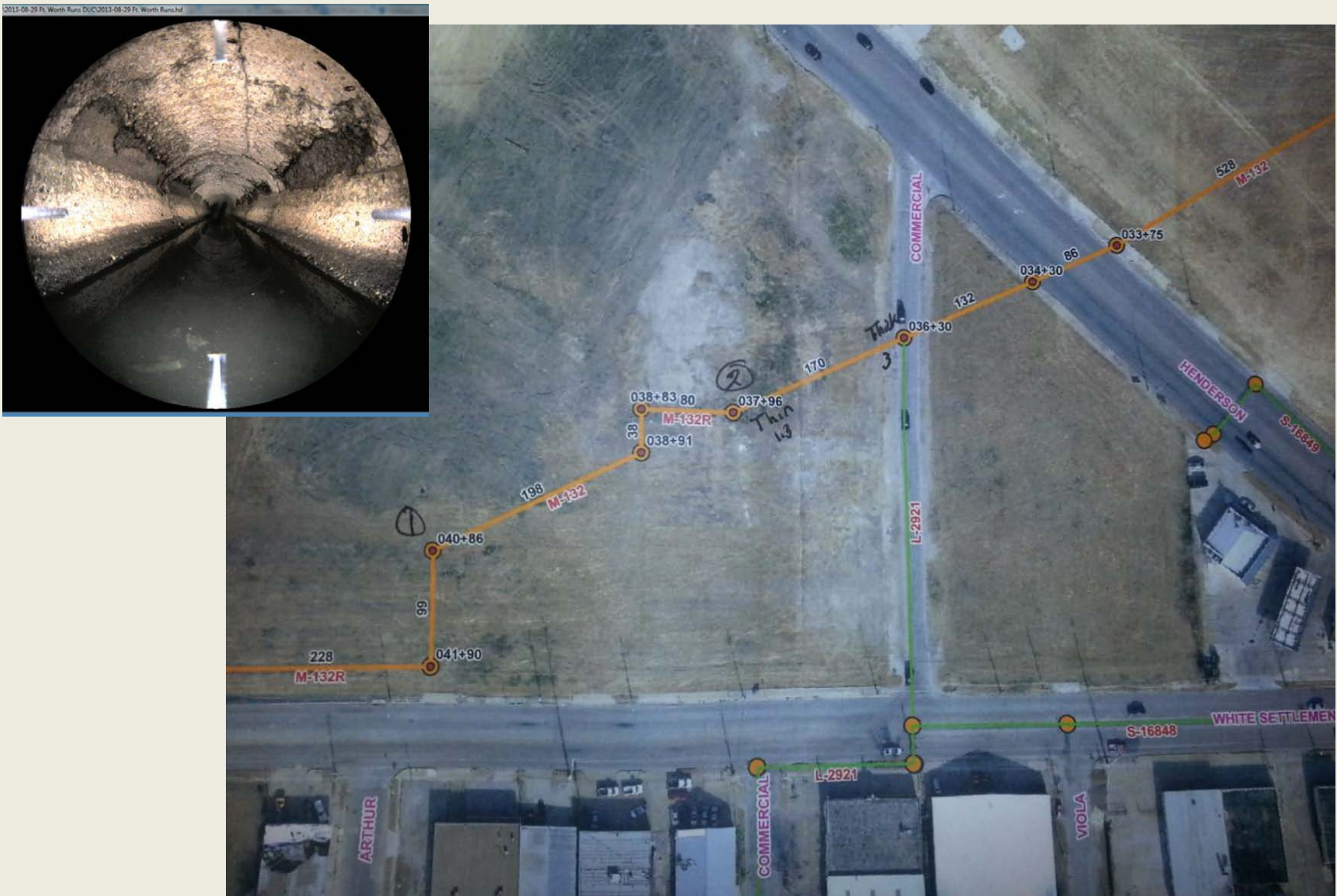
Ft. Worth Pipe Wall Thickness Measurment 24" deteriorated RC Sewer line
