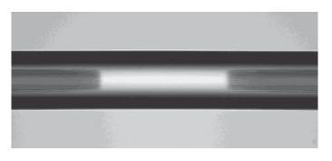
Collapsed region (bright in center) of fiber, with photonic crystal holes visible to left and right of collapsed region (optical microscope image).
