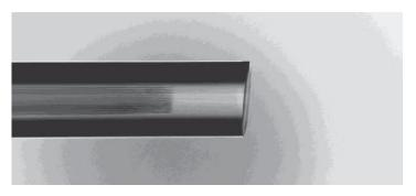
Angle-cleaved fiber showing typical size of remaining collapsed region (optical microscope image).
