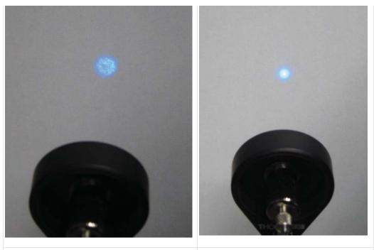
Speckle mode - note larger diameter/beam spread and speckled quality. Very sensitive to fiber jiggling.
