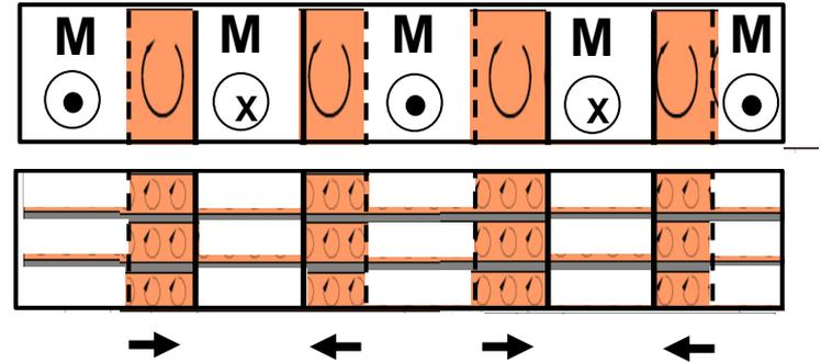
Increase Domain Wall Density to Minimize Wall Velocity and Reduce Localized Losses
