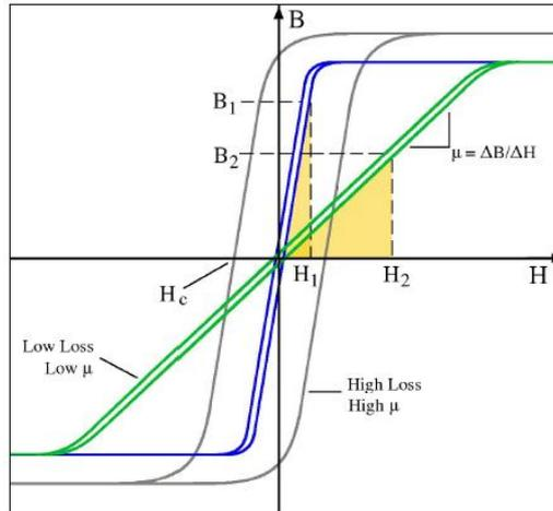
For Bulk Alloys Grain Boundaries and Precipitates Act as Pinning Sites Increasing Losses
