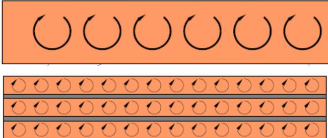
Laminate Structure with Reduced Thickness and Select High Resistivity Materials
