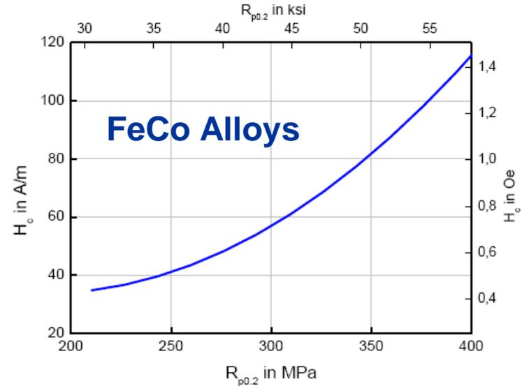
Figure 2: Possible combinations of coercivity  $H_c$  and yield strength  $R_{p0.2}$  for VACODUR<sup>®</sup> 49.
