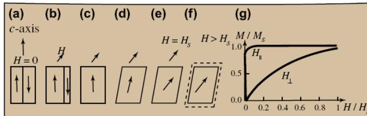
**Figure 23** Steps in the magnetization process (a) virgin state, (b) wall motion, (c) monodomain, (d) rotation, (e) saturation and application of a field exceeding that required to saturate. (For color version of this figure, the reader is referred to the online version of this book.)
