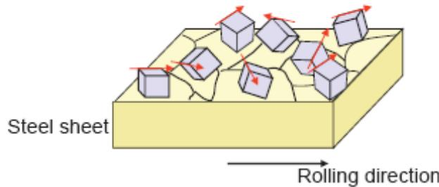
It's desirable to have as many (100) plane as possible, including the axis of easy magnetization. It's vital to minimize (111) plane.
