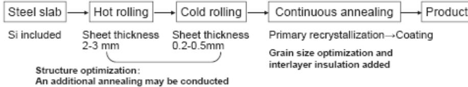
Non-oriented electrical steel sheet products = Primary recrystallized structure
