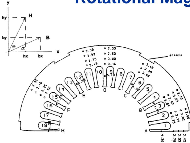
Localized loss (W/kg) at various points in the annealed core at 1.0T in stress free condition.
