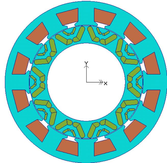
*Schematic of internal permanent magnet motor*
