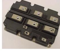
Si IGBT Switching Frequency Capability Decreases Rapidly with Voltage Rating Due to Increased Losses
