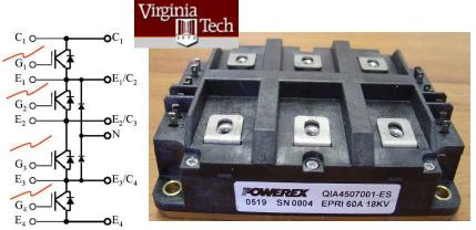
4.5 kV, 60A IGBT (3-Level diode-clamp)
