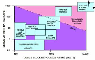
New Switch Capabilities enables new Applications Hi-T, Hi-Rad, Hi-V, Hi-f
