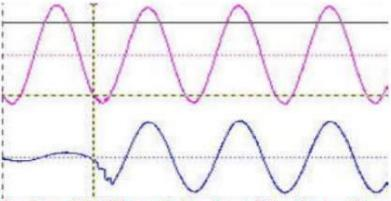
Top View: EPCC Output Voltage Sag (~5%) w/ System Motor Load Surge Current Bottom View: ~ 50HP Motor Inrush Surge Current on EPCC Output
