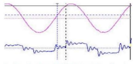
Top View: Non-Distorted EPCC Output Voltage Waveform Bottom View: Identical Non-Linear Load Current at EPCC
