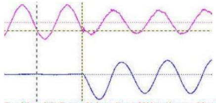
Top View: DG Output Voltage Sag (~35%) w/ System Motor Load Surge Current w/o EPCC Unit Bottom View: ~50HP Motor Inrush Surge Current on DG
