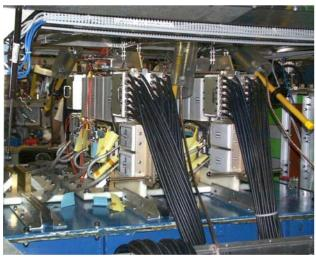
20 KHz IGBT Switching Assemblies
