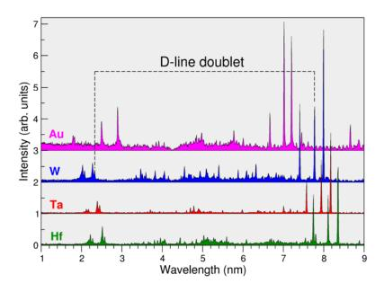
Figure 4.1: Measured soft x-ray spectra from highly-charged ions of Hf, Ta, W, and Au. The D-line doublet for sodium-like W<sup>63+</sup> is shown by dashed lines.
