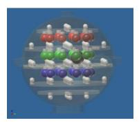
Figure 1 Solid model of MRI system phantom
