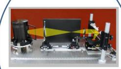
Versatile detector systems for passive THz imaging.
