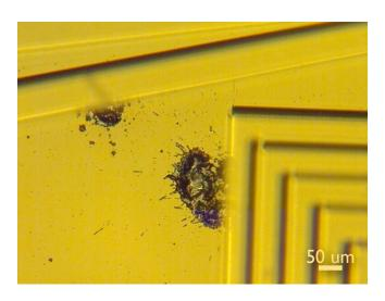
Figure 8.23: The micrograph shows evidence of breakdown on a SOI structures due to charging in the Plasma Ops III oxide etcher.
