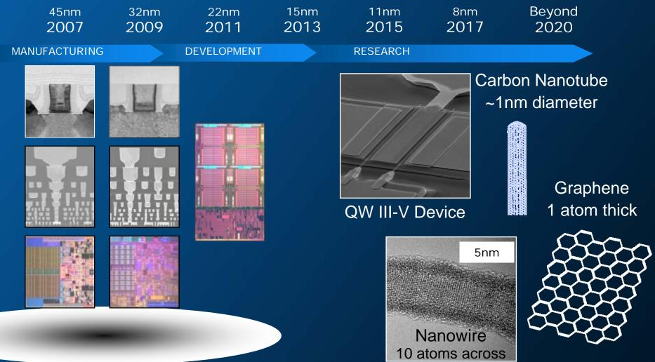
Silicon lattice is ~ 0.5nm, hard to imagine good devices smaller than 10 lattices across – reached in 2020
