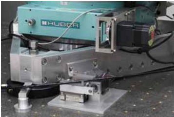
Spherical air bearing base for CDPBD
