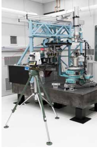
CDPBD during alignment on granite base
