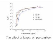
provided an experimental comparison with 2D percolation theory. It also showed that sorted nanotubes, even of a shorter average length, may perform better than unsorted tubes due to their tendency to pack in a 2D (rather than a 3D) network.
