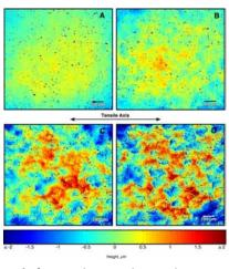
Surface roughness evolution with strain
