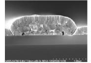
The CdTe grains coarsen during annealing
