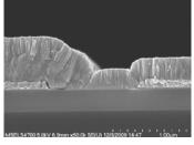
A photovoltaic with CdTe on one platinum electrode with ITO over the entire device.
