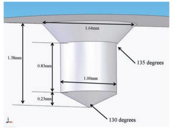
form various angles, useful for hip arthroplasty procedures (See Exhibits 8 and 9). An arc at the base of the coordinate frame has been fitted with target holes spaced at regular angular increments, offering additional angular calibration and testing capability (See Exhibit 10). The magnetic ball and socket joint are commercially available and made of stainless steel, while the
