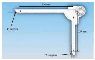
exhibit) and  $Y_1$  to  $Y_{15}$  on the Y axis (vertical in the exhibit). The nominal incremental distance between these target points is 15 mm, which gives a nominal X axis length of 300 mm and nominal Y axis of 225 mm (See Exhibit 8). The X axis is longer because it is intended to approximate the length of an adult femur bone. The distance between any two target holes is measured between the tips of the two holes. Although the
