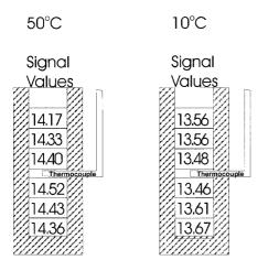
Fig. 3. Dependence of the EPR responses of alanine dosimeters on their position in a polystyrene vial with a thermocouple inserted in the vial center. The vials with the dosimeters were kept at the specified temperatures for 45 min, the subsequent irradiations to 10 kGy took about 1 h.
