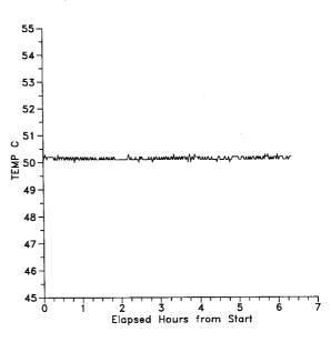
Fig. 4. Variations in the temperature of the thermostatted aluminum during the 1.25-h pre-irradiation period and 5-h irradiation at a dose rate of 9.5 kGy/h.
