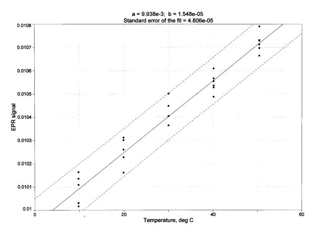
Fig. 2. A typical plot of the alanine dosimeter response on irradiation temperature using Bruker dosimeters (dose 13 kGy). Some of the closely positioned points are not resolved. The dotted lines show the prediction band; no outliers occur in this experiment.
