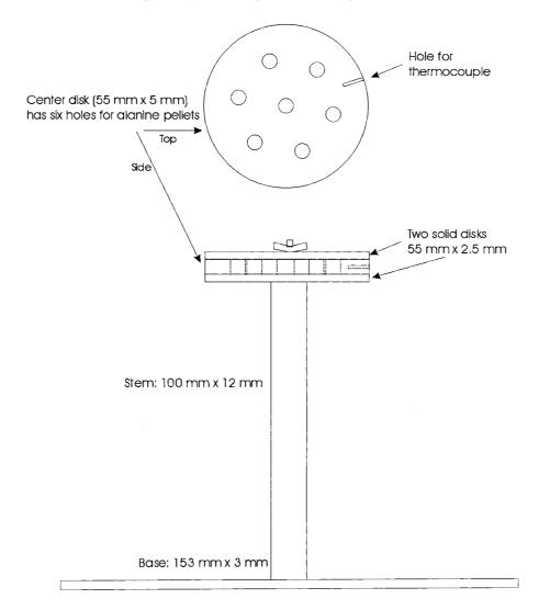
Fig. 1. Aluminum holder used for dosimeter irradiation at controlled temperatures.
