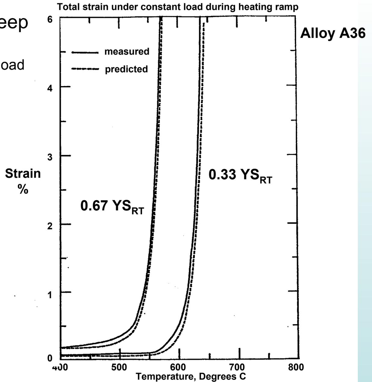
Figure 11. Measured and predicted strains during a non-linear heating rate for stresses of 1/3 and 2/3 of the room temperature yield strength.
