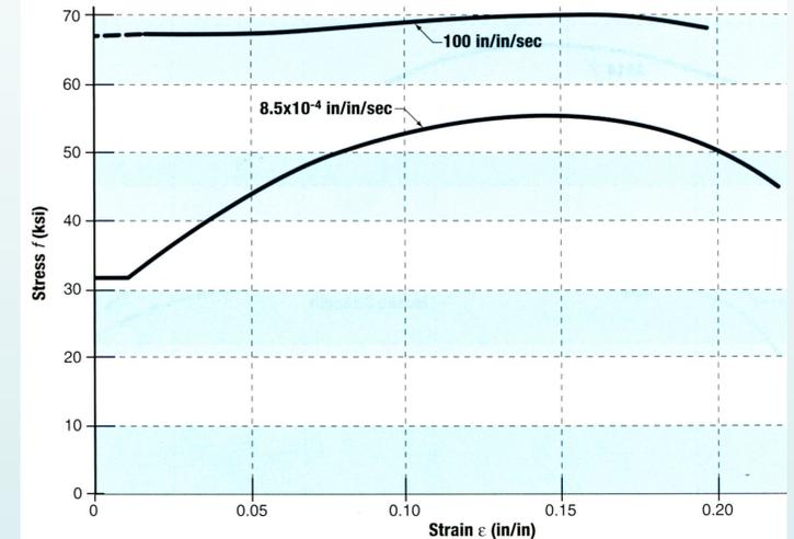
Figure B-4 Effect of high strain rate on shape of stress-strain diagram (Tall 1974).
