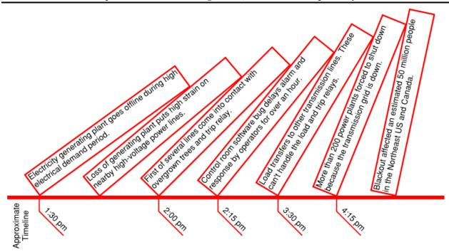
Figure 4-3: Power System Internal Dependence Cascading Failure in the 2003 Northeast Blackout
