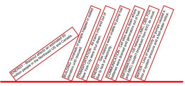
Figure 4-4: External Dependence Cascading Failure in the 2003 Northeast Blackout
