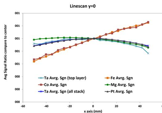
LEXES can **detect and quantify all the elements** of the stack with quite good repeatability.
