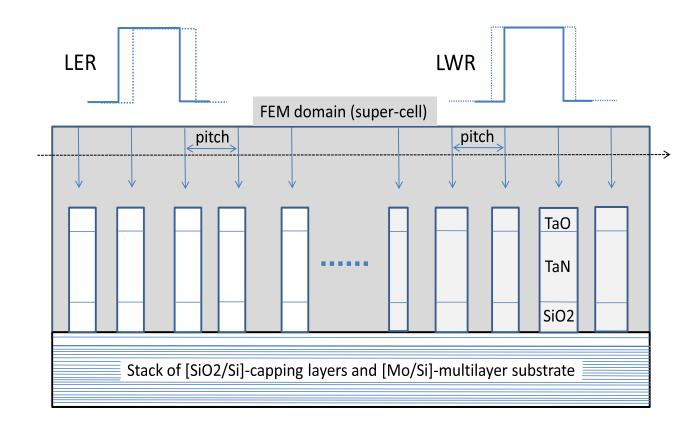
FIGURE 1: Profile model used for line edge (LER) and line width (LWR) roughness in a large FEM computation domain: randomly changed center positions for LER (left) and randomly changed line widths for LWR (right) are superimposed independently to create LEWR perturbations. normalized deviations can be approximated by
