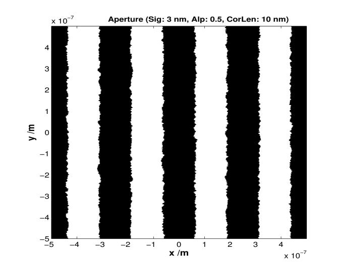
FIGURE 2: Aperture model used for 2D Fourier transform approach: Roughness of the edges of the aperture slits is provided by a power spectrum density function, which depends on a standard deviation, a correlation length and a roughness exponent.
