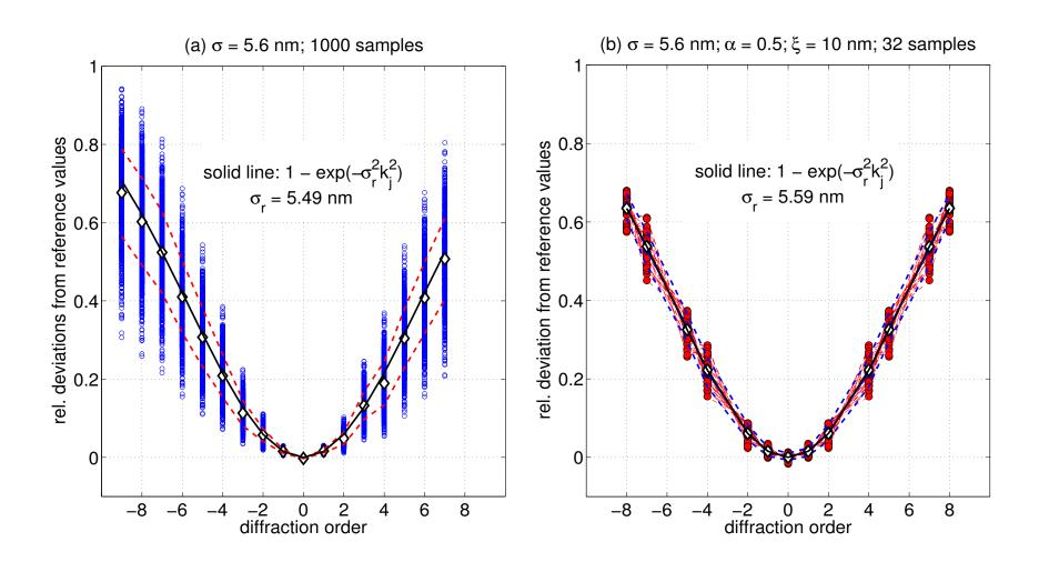
FIGURE 3: Normalized deviations from the efficiencies of the unperturbed reference line structure (for two examples), depicted as circles; diamond symbols represent the mean deviations of all samples; dashed lines indicate the mean efficiency  $\pm$  standard deviation; solid lines depict the exponential approximation; (a) for FEM simulations and (b) for 2D-Fourier simulations of a binary grating.
