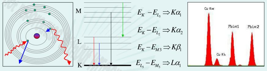
• Incident x-ray via photoelectric interaction knock out electrons from innermost atomic shells.
