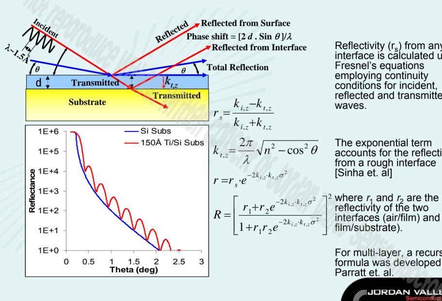
Reflectivity (r<sub>s</sub>) from any interface is calculated using Fresnel's equations employing continuity conditions for incident, reflected and transmitted waves.
