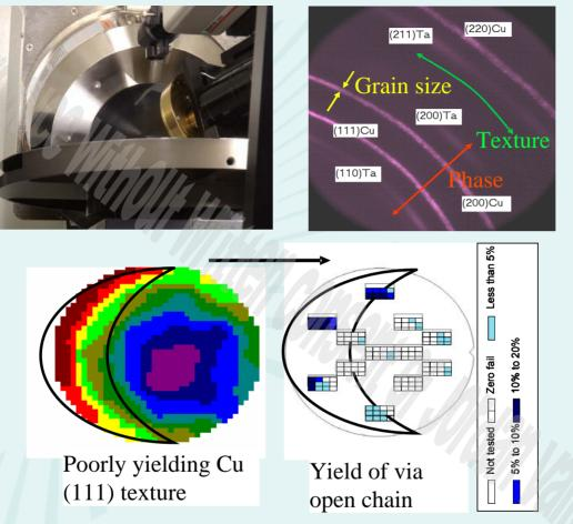
Cu Texture, i.e., non-random or preferred orientation of crystallites analysis of post-polish Cu establishes correlation of yield loss.
