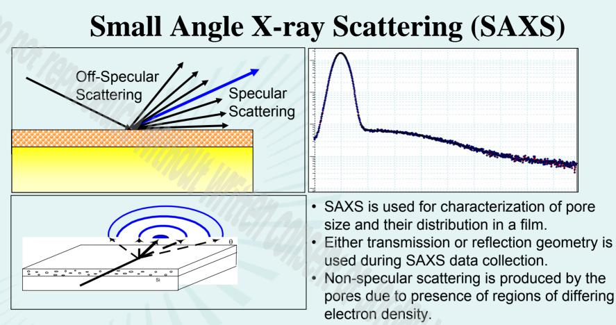
For randomly distributed pores, the scattering intensity as a function of Bragg size "d" or "r" is proportional to the number of scattering elements in the irradiated volume and its atomic scattering factor.
