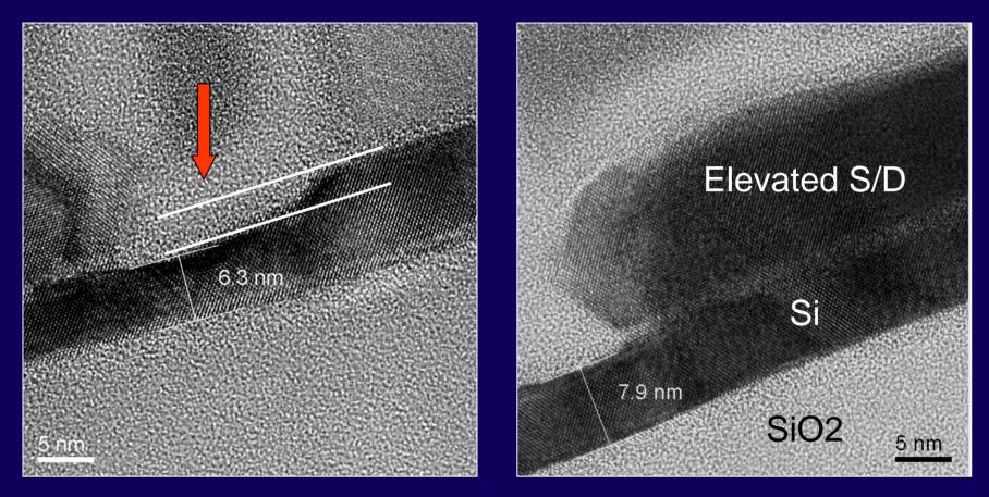
Excessive Silicon etching during surface cleaning steps may influence channel characteristics
