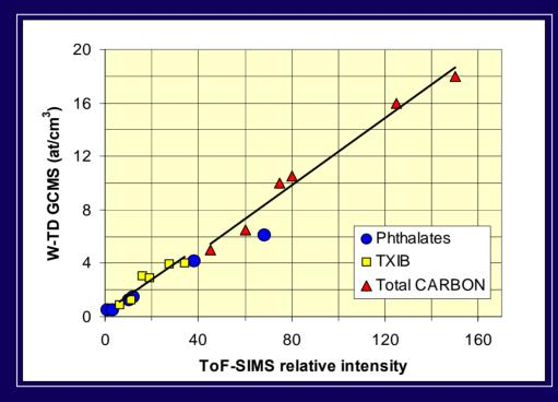
At Room Temperature ~ 30 – 70 % of the volatile species desorb from the wafer surface and remain undetected by ToF-SIMS!
