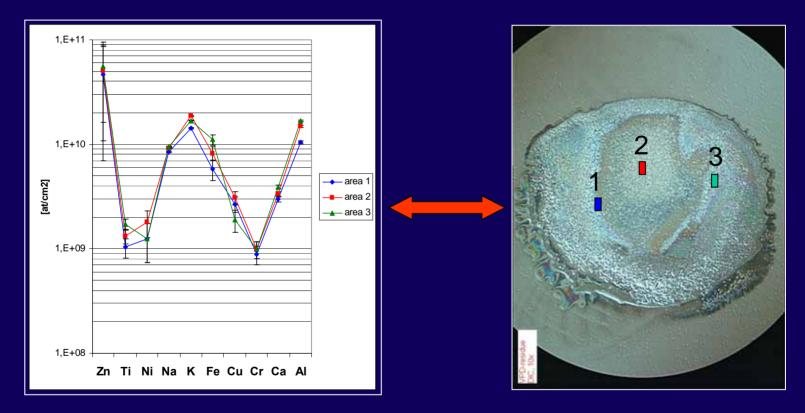
ToF-SIMS analysis (left) at different locations within the droplet (right) shows its constant chemical composition
