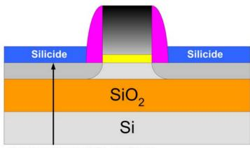
Solution: Elevated Source/Drain
