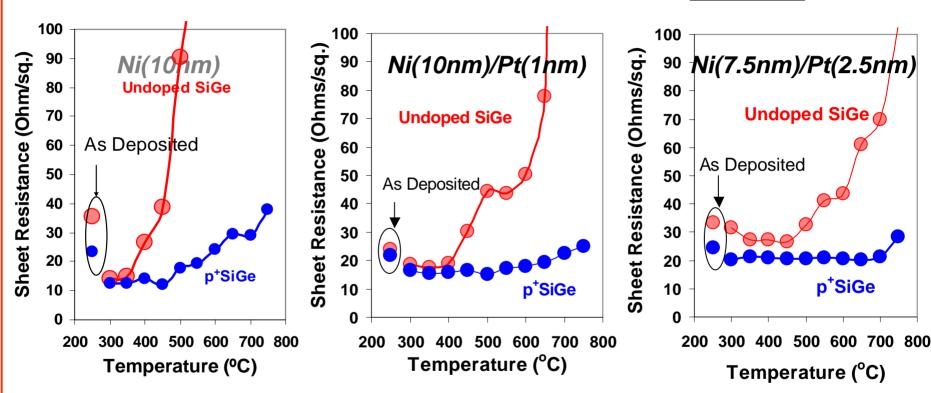
Sheet resistance thermal stability greatly improved On p<sup>+</sup> SiGe - sheet resistance of Ni(7.5nm)/Pt(2.5nm) is stable up to 700°C
