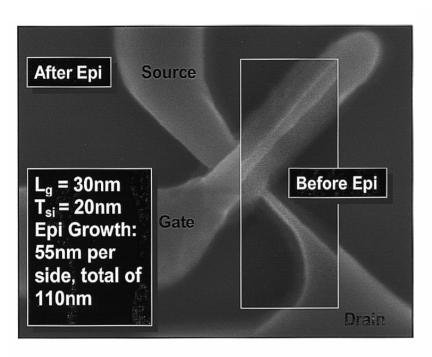
Fig. 7. Top down SEM micrograph, of  $\langle 100 \rangle$  FinFET before and after selective Si epitaxy. Device measurements:  $T_{\rm si}=20$  nm,  $L_{\rm poly}=30$  nm, 55 nm of silicon was grown selectively on each side of the fin.
