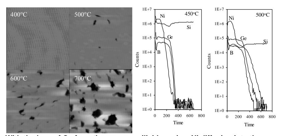
With the loss of Ge from the germanosilicide grains, Ni diffusion into the underlying SiGe results in NiSi spikes that extend deep into the substrate
