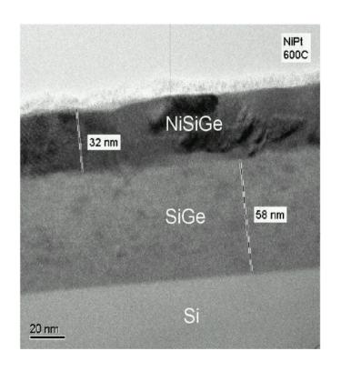
RMS Interface Roughness ~ 1 nm
