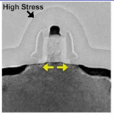
Fig. 3 TEM of NMOS transistor showing high tensile stress nitride overlayer. PMOS: uniaxial compressive stress from sel. SiGe in S/D
