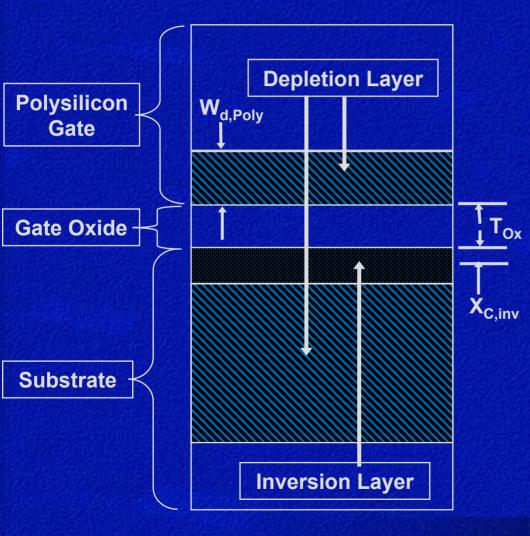
(W<sub>d,Polv</sub>+X<sub>C,inv</sub>)  $-K_{ox} = 3.9$  $-K_{ei} = 11.9$ • $T_{ox,electric} = T_{ox} + (0.33)^* (W_{d,Poly})$ +X<sub>C,inv</sub>) -W<sub>d,Poly</sub>~1/(poly doping)<sup>0.5</sup> →increase poly doping to reduce W<sub>d.Poly</sub> with scaling -But max. poly doping is limited→can't reduce W<sub>d.Polv</sub> too much -Fermi Level pinning with highk •Poly depletion and X<sub>C.inv</sub> become more critical with Tox scaling -Eventually, poly will reach its limit of effectiveness
