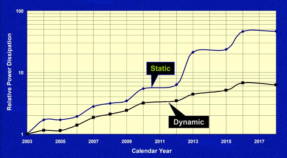
Assumption, to make a point re P<sub>static</sub>: all transistors are high performance, low V<sub>t</sub> type
