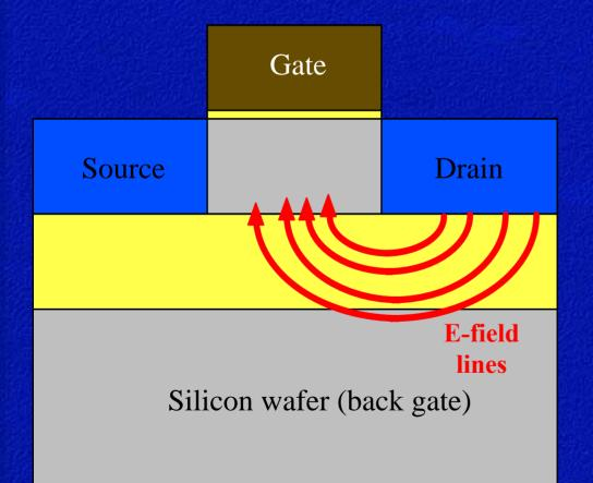
**Electric field lines** from the drain encroach on the channel region. Any increase of drain voltage decreases the threshold voltage (the "NPN" potential barrier between source and drain is low
