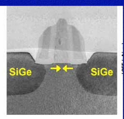
Fig. 4 TEM of PMOS showing SiGe heteroepitaxial S/D inducing uniaxial strain.
