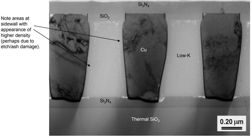
Conventional Bright Field TEM image of completed M1 test vehicle incorporating Low-K **after TC1** (400°C, 1 hr.) anneal.
