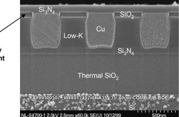
XSEM image (FIB/BOE) of completed 0.35µmL/0.40µmS COMB structure **after TC2.**
