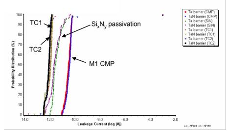
Leakage current probability plot for 4 sequential etest steps.
