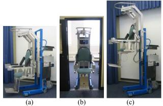
Figure 2 – Photographs of the HLPR Chair in the mobility configuration showing the (a) side view and (b) front view relative to a typical doorway and (c) the lift configuration. The maximum patient lift height is 0.9 m (36 in) above the mobility height configuration.
