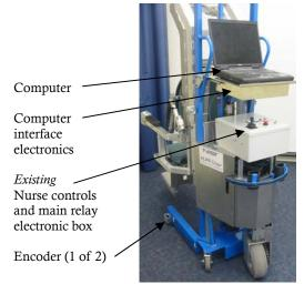
Figure 6 – Photograph of the HLPR Chair with recently added front wheel encoders, development computer and interface electronics, and advanced 3D imaging camera and color camera (cameras are shown in Figure 1).
