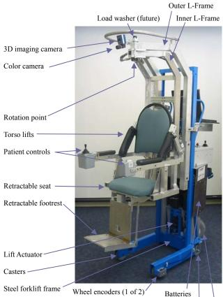
Rear Casters (only for anti-tip) Drive/Steering motors and wheel
