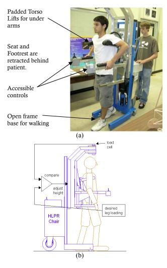
Figure 8 – (a) Photograph of the HLPR Chair prototype in the rehabilitation/walking configuration. Summer Interns (Alex Page and Robert Vlacich) demonstrate the
