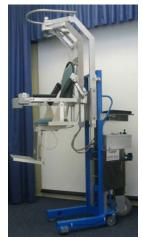
Figure 3 – HLPR Chair prototype shown in the patient lift position.
