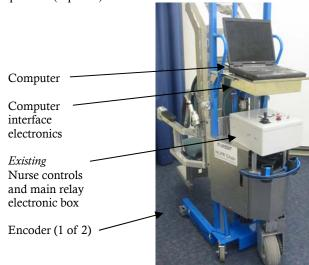
Figure 6 – Photograph of the HLPR Chair with recently added front wheel encoders, development computer and interface electronics, and advanced 3D imaging camera and color camera (cameras are shown in Figure 1).
