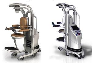
Figure 9 – Front (left) and rear (right) concept drawings of the HLPR Chair as a more ergonomic and commercialized version.
