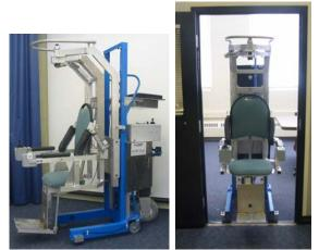
Figure 2 – Photographs of the HLPR Chair in the mobility configuration showing the side view (left) and front view relative to a typical doorway (right).
