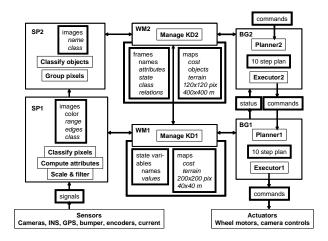
Figure 7 – NIST 4D/RCS 2-level, hierarchical control architecture developed for the DARPA LAGR Project and planned for implementation on the HLPR Chair.
