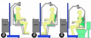
Figure 4 – Graphic showing the concept of placing a patient onto a toilet or chair with the HLPR Chair. The patient drives to the target seat (left), manually rotates near or over the seat (middle) while the torso lifts support the patient and the seat retracts, and then is lowered onto the seat - toilet, chair or bed (right).
