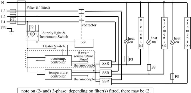
or) 3 separate neutral wires from the elements to the neutral supply.
