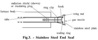
the end of an extended work tube they can increase the bending stress at the centre of the tube. Support such fittings in such a way that expansion of the tube is allowed.
