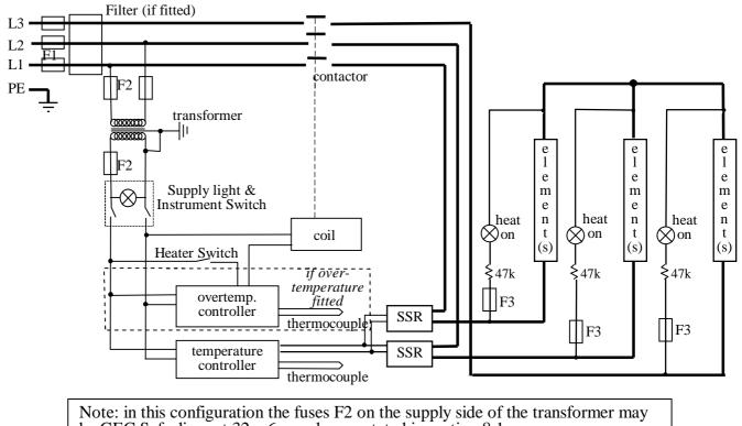
be GEC Safeclip, not 32 x 6mm glass as stated in section 8.1.
