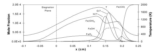
FIGURE 3: Iron species, O, H, and temperature with 200 ppm inhibitor in the air, near extinction (a= 257 s<sup>-1</sup>). The stagnation plane is noted by the line at x = 0.  $x_f = -0.4$  cm,  $x_{air} = 0.6$  cm.
