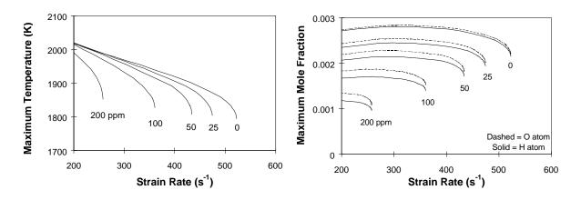
FIGURE 4: Maximum flame temperature vs. strain rate for  $X_{in}$  between 0 and 200 ppm.
