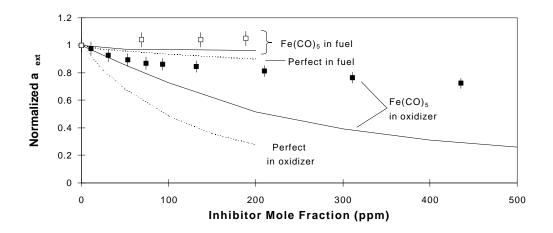
FIGURE 2: Normalized extinction strain rate for counterflow diffusion flames. Closed symbols: measurements with the  $Fe(CO)_5$  in the oxidizer; open symbols: measurements with  $Fe(CO)_5$  in the fuel; solid lines: calculations with  $Fe(CO)_5$ ; dashed lines: calculation with perfect inhibitor. Data from Ref. [5].
