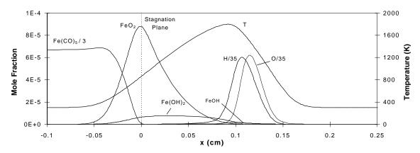
FIGURE 8: Iron species, O atom, H atom, and temperature for flame on the air side, 200 ppm inhibitor in the fuel, near extinction (a = 496 s<sup>-1</sup>). The stagnation plane is noted by the line at x = 0.  $x_f = -0.4125$  cm,  $x_{air} = 0.5875$  cm.
