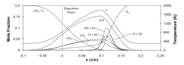
FIGURE 1: Calculated flame structure for a CH<sub>4</sub> vs. air flame near extinction ( $a=522 \text{ s}^{-1}$ ). The stagnation plane is noted by the line at x = 0. Fuel jet location ( $x_f$ ) = -0.41 cm, air jet location ( $x_{air}$ ) = 0.59 cm.
