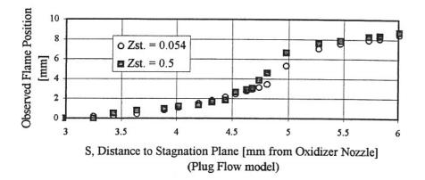
Figure 3. Variation of Observed Flame Position with the parameter S.
