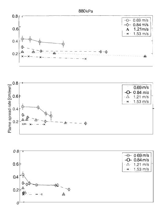
Figure 7. Flame spread rate as a function of surface loading for 6.4 mm thick PMMA.
