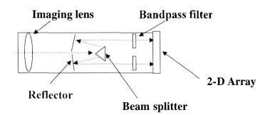
Figure 3. Schematic of the two color planar pyrometer.
