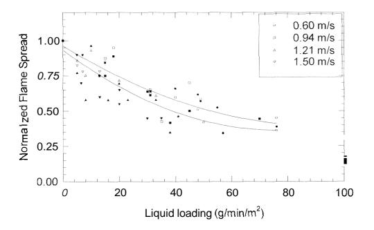
Figure 9. Variation in normalized flame spread with liquid loading.
