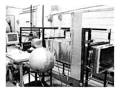
Figure 1. Wind tunnel used for fire spread studies.
