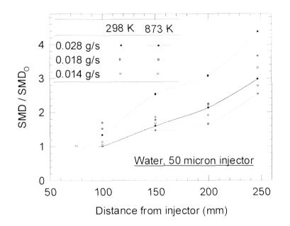
Figure 17. Change in SMD of the droplets with axial distance for water.
