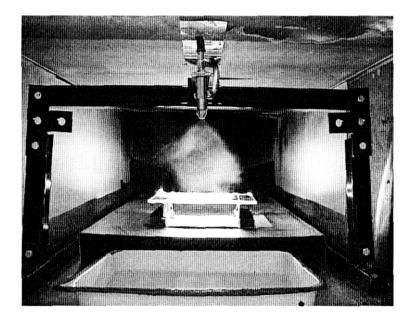
Figure 2. Flame spread experiment with water mist.
