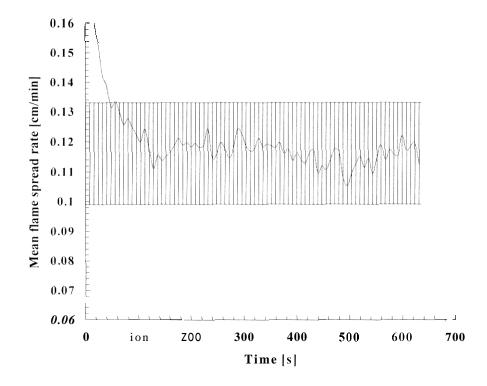
Figure 4. Typical flame spread time trace obtained using Focal Plane Array Imaging.
