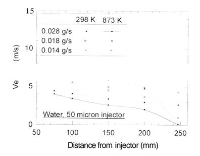
Figure 19. Variation in velocity with axial distance for water spray
