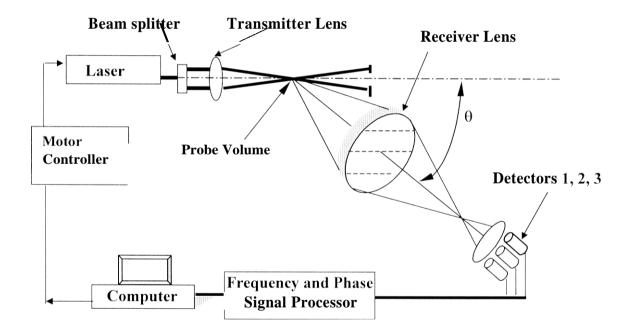
Figure 15. Schematic diagram of PDPA instrument
