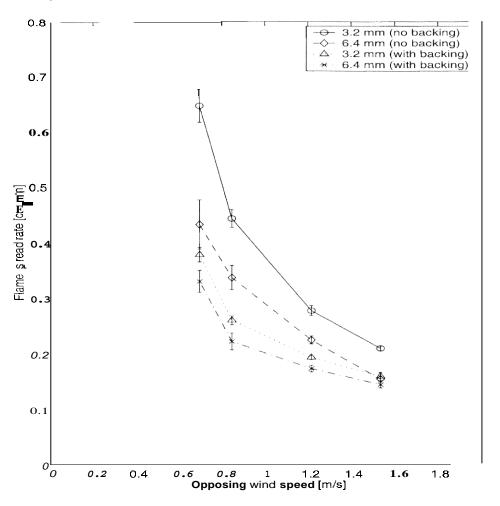
The flame spread rate as a function of opposing wind speed is shown in Fig. 5. The vertical bars represent one standard deviation in the statistical variation of the data on
