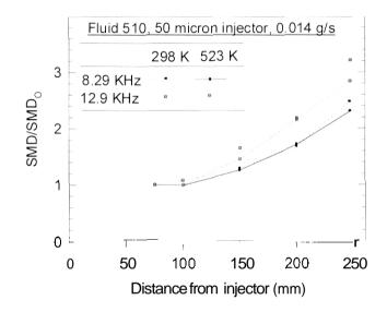
Figure 18. Change in SMD of the droplets with axial distance for Fluid 510
