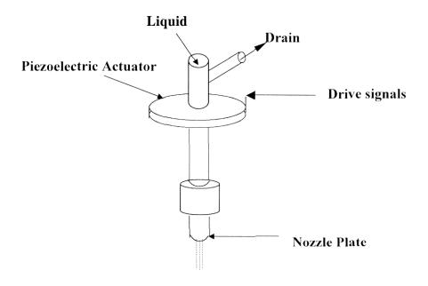
Figure 12. Configuration of the piezoelectric atomizer
