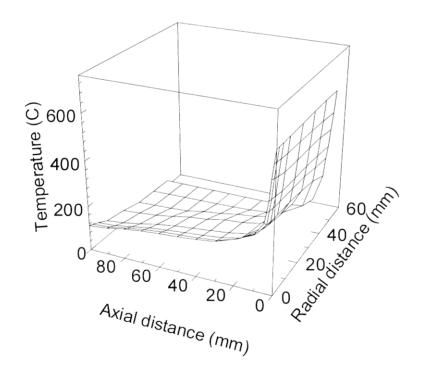
Figure 16. The temperature field at steady state above the hot plate
