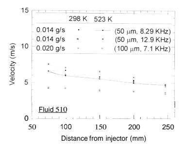
Figure 20. Variation in velocity with axial distance for Fluid 510.
