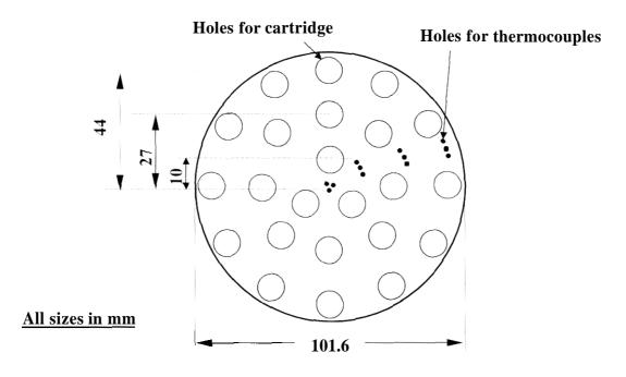
Figure 14. Temperature measurement locations on the heater
