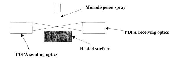
Figure 11. Experimental arrangement for the PDPA measurements
