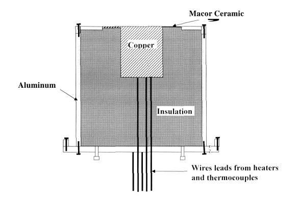
Figure 13. Schematic diagram of the heater assembly
