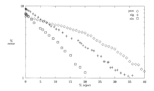
Figure 4: Error reject graph for sigmoidal MLP, sinusoidal MLP, and PNN for classification of fingerprints.
