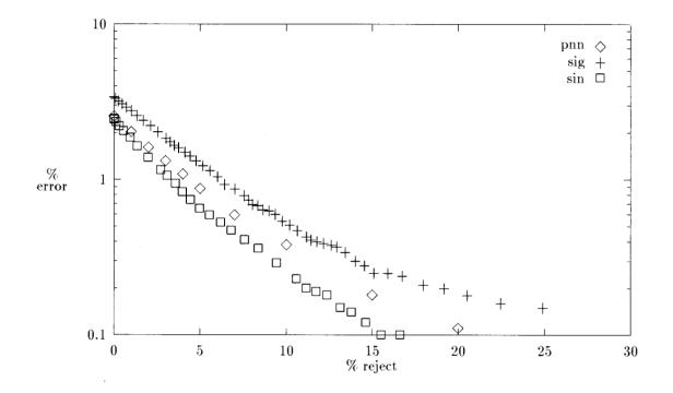
Figure 3: Error reject graph for sigmoidal MLP, sinusoidal MLP, and PNN for classification of digits.
